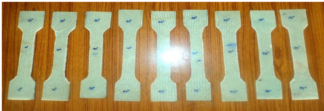
Fig 2: The specimens with different orientations are prepared for tensile test
